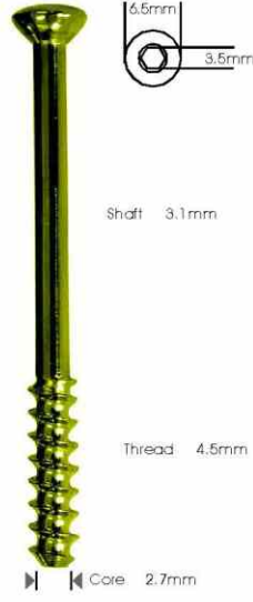
CORTEX CANNULATED SCREW 4.5MM SHORT THREAD
