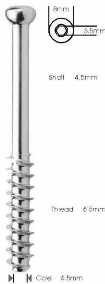
CANCELLOUS CANNULATED SCREW 6.5MM - 32MM THREAD
